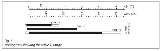
$K_v$  values are always given for water flow in  $[m^3/h]$  with a pressure drop  $\Delta p$  of 1 bar. The valve should be selected so that the necessary  $k_v$  value lies in the middle of the regulation range.
