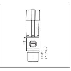
The valves can be installed in any position. An arrow on the valve body indicates the direction of flow. FJVA valves are also marked so that the letters RA can be read straightforwardly. The installation of an FV filter ahead of the valve is recommended.
