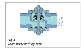
FJVA valves are for applications where, because of installation problems, etc., it is desirable to avoid using a capillary tube. This applies mainly where regulation accuracy requirements are more moderate and where an integral bypass can be accepted.
