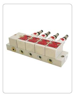
Flow limiters are used in large oil circulation lubrication systems. The task of a flow limiter is to divide up the volumetric flow of the main line into parallel individual volumetric flow quantities and to "limit" these according to requirements, or to keep them constant. The volumetric flow generated is independent of the system pressure and nearly independent of viscosity.
