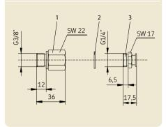
Filling device with quick-action coupling
