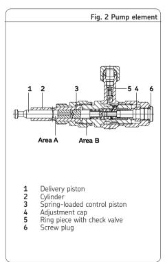
Delivery volume adjustment on pump element- see Figures 2 and 3
