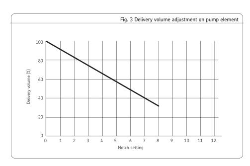
Delivery volume as a function of the notch setting on the pump element for piston diameters 6 mm, 8 mm and 10 mm
