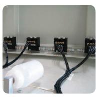
running, automatic lubrication systems reduce friction inside bearings and help prevent contamination. The result is optimized bearing service life over the long term, more turbine uptime and reduced manpower costs – all combining to help make wind farms more profitable.
