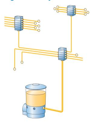
In progressive automatic lubrication systems, a piston pump supplies a defined amount of lubricant through the main line to the metering device that serves each outlet.
