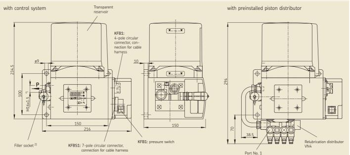
\*) Ports tapped for solderless tube connection for 10 mm diam. tube.
