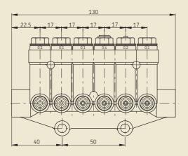
Quick connector connection for 4 mm diam. plastic tubing.
