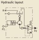
P1 = air line from compressed air network P2 = main line of system
