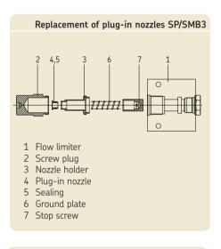
Replacement of plug-in nozzles SP/SMB6
