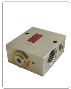
The SP /SMB3 and the SP/SMB6 flow limiter comes with two throttles installed in series  $(D_1, D_2)$ . Throttle  $D_1$  is an interchangeable plug-in nozzle which, as a nonadjustable orifice, determines the rated volumetric flow. Nonadjustable orifice  $D_1$  is available with different nozzle cross sections (see tables on pages 8 and 10).
