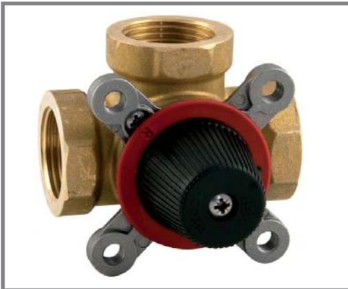
A 3-way mixing valve mixes heating water for a heating system to a required temperature. Mixing is done by a circular segment rotor. The rotor turning angle used for regulation is about 90° and corresponds to a scale from 0 to 10 (without stops it can rotate 360°).
