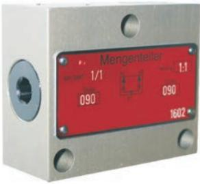
Flow dividers used in SKF CircOil lubrication systems separate the volumetric flow of the main line into parallel individual volumetric flows and limit these according to demand. Sensor or gear-type flow indicators are used to monitor the volumetric flow. They provide an almost constant flow rate due to pressure-compensated technology, regardless of oil viscosity and pressure changes.
